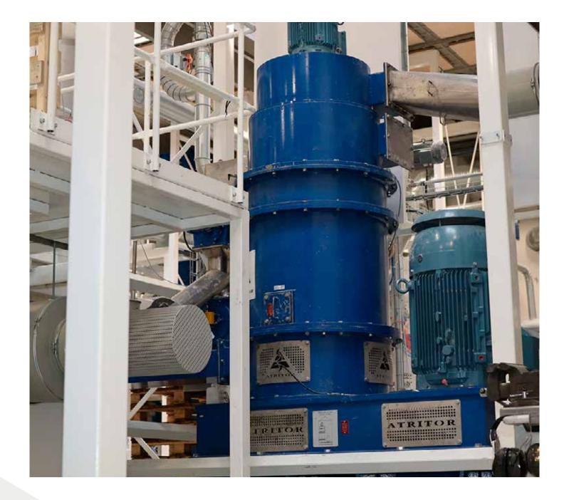
Freebee approached three suppliers to assess their technology and after extensive testing, the Atritor Cell Mill was chosen. This was due to the simplicity of blade design, in addition to Atritor's collaborative approach. The integral blade design in the Atritor mill provided a better overall performance than offered by the alternatives.
